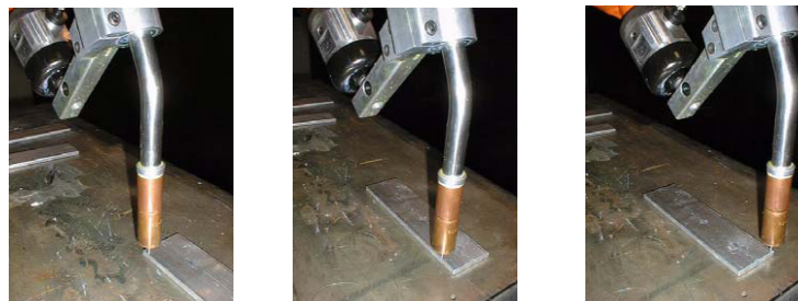
Figure 4-2 Movement of robot arm and torch with correct TCP
