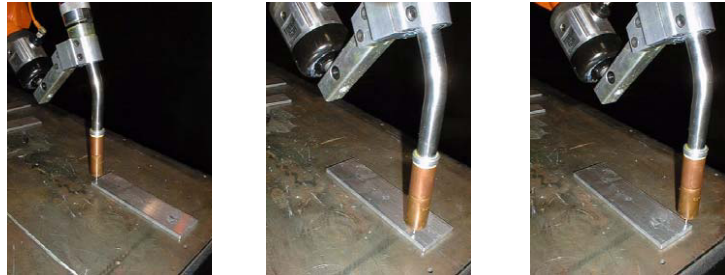
Figure 4-3 Robot arm moves on the same trajectory, however the torch trajectory has changed
